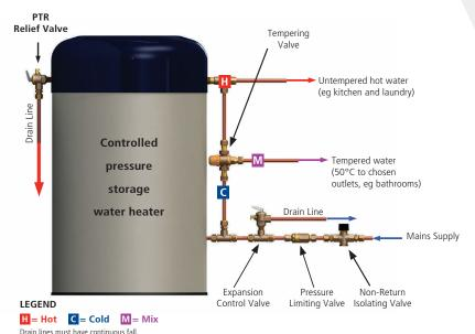
The TCV is factory set at 65°C. If required to be used as a safety valve, the TCV must commissioned on site to no more than 50°C by licensed plumber as per AS3500.
