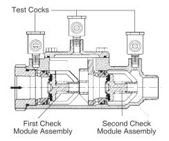
The 007 Series features a modular design concept which facilitates complete maintenance and assembly by retaining the spring load.
