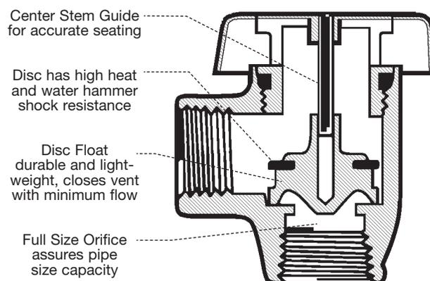
Since atmospheric type vacuum breakers are subject to normal maintenance and replacement, they should be located where emergency water spillage will create no problem and where they can be accessible for inspection or servicing.
